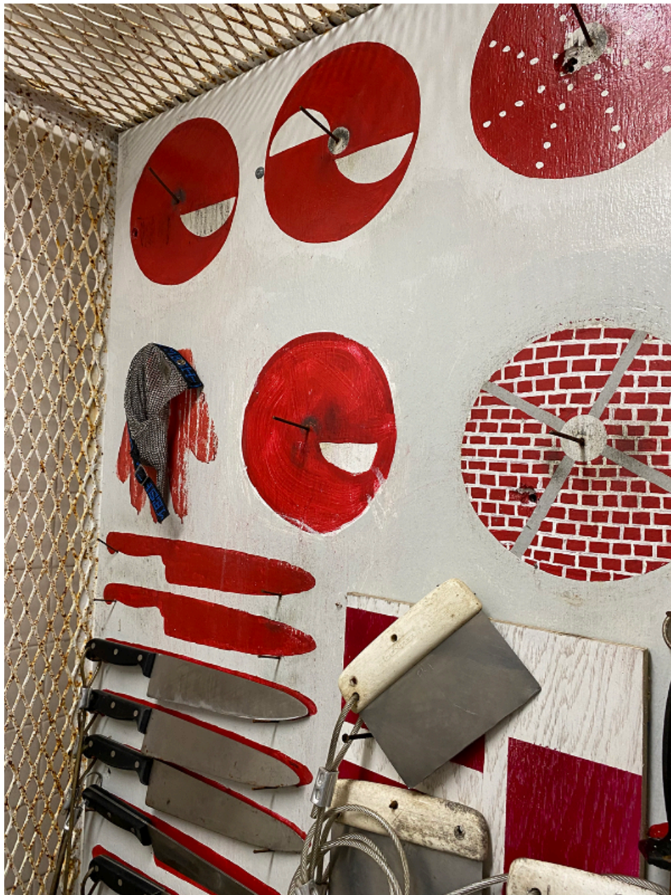
Knife Box Shadow Board With Missing Tracking Markers for Two Knives and Five Other Sharp Tools. Source: OIG, June 2024
