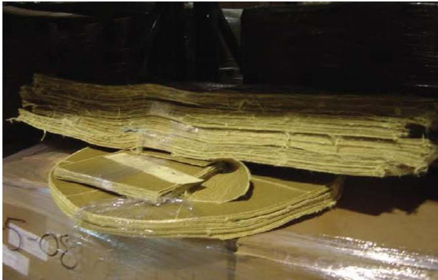
**Figure 3. Kevlar bonded together.**
